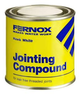
Hawk White is a pipe jointing compound for use in general applications. It is suitable for Natural Gas, non-potable water, steam, air (excluding medical lines) brine, alcohol and L.P. Gas. It is ideal for use on pipe diameters up to 25mm and with reinforcement fibre on pipework over 25mm.
