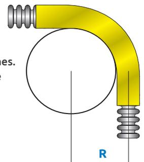
**Do not bend / unbend tubing multiple times. Tighter bend radius will increase pressure drop, please adhere to above guidelines**
