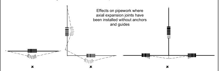
Anchors and pipe guides are essential to ensure the correct performance of the axial expansion joints. Ensure that only one axial expansion joint is installed between anchors.
