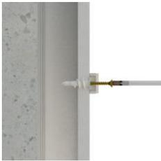
**2. SET THE FIXTURE AND INSTALL THE SCREW**
