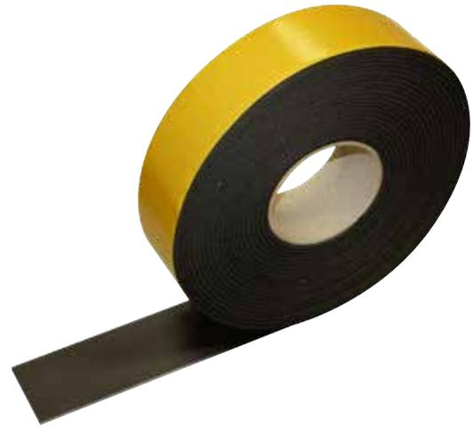
Highly flexible closed cell elastomeric foam (FEF) suitable for hot and cold thermal insulation, featuring a combination of low thermal conductivity, high water vapour diffusion resistance and low flame spread.
