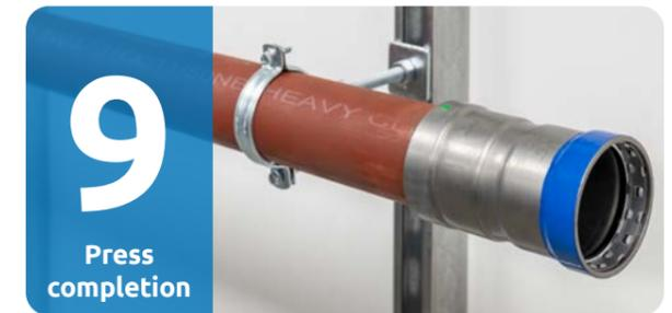
Inspect the assembly after completion of the press to confirm correct completion. The pipe insertion mark should be double checked for position at the fitting edge, to ensure that full engagement has been maintained. The plastic foil indicator will have become detached, and any remains of this can be removed so the fitting is left clean and visible as a completed joint.
