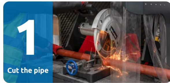
Cut the suitable steel pipe to the required length using an appropriate tube cutter to ensure a clean, square cut. Suitable tools include a proprietary pipe cutter, powered saw with the correct toothed blade for the material and a hacksaw with a fine-tooth blade.
