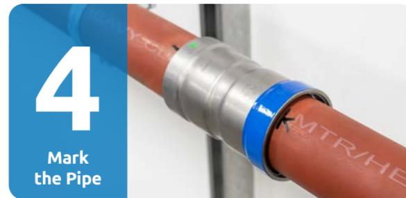
Mark the correct insertion depth clearly onto the pipe surface (or the fitting for m x f fittings) using a marker pen or similar. Mark the edge position of the fitting to enable easy visual checking that the tube has not moved prior to or during the press operation. It is critical to ensure that correct engagement has taken place.
